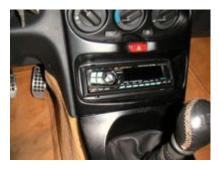
This surround does not affix itself to the aperture, it relies on the new stereo cage to hold itself in place. Whilst this works, it will rattle. When you fit this piece take the time to smear the back of it with silicon sealant to ensure that it won't rattle once you have your new head unit installed.
