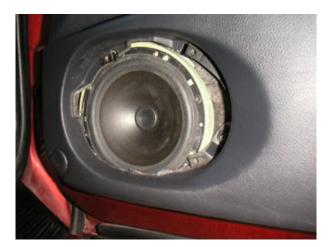
That's it! Your front speakers are fitted, now you have 6.5" component speakers in the front and the back of the car! Replace the grilles (you will have to remove the lower mounting clip) and you wouldn't even know they were there.  $\underline{\mathbf{y}}$
