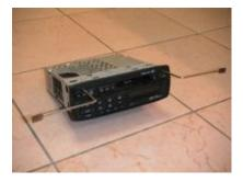
On the back of the unit you'll find some connectors, unclip these and pull out the aerial plug. Put the stereo to one side and look back into the slot where it once sat. You should see a metal "cage" protruding into the empty hole from the edges of the slot. This is held in by pushing out metal cutouts on the cage, these cut-outs lodge themselves behind the dashboard so the cage (and the stereo) won't fall out.
