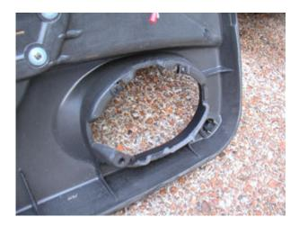
As you can see, the section in the lower corner needs to be cut back to the same level as the speaker grille clip holders. Whilst this does mean cutting off one door card mounting point, don't worry, you don't need it! It won't make your door card loose when refitted, nor will it create any extrs rattles.
