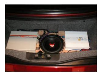
You will want to finish things off now. Once all the electronics are all set up properly, mount some MDF or wood blocks onto the sub enclosure that come up to the same height as the tops of the two intruding sub-frame/rear bumper mount points at the back of the boot. In fact, if you find that your sub box is moving about in the boot, you can mount the box to these two metal parts.
