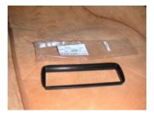
Make sure you fit this item now, if you want to fit it at a later date you will have to remove the stereo again! It is worth the hassle though, for a little piece of plastic, it makes a huge difference to the overall look of the installed head unit.
