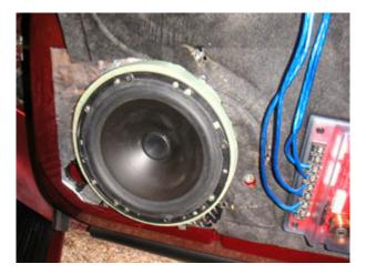
Finally, you will need to fit the crossover units. The best place for these is on the door, mounted just behind the gap that sits between the grab handle and the door pocket on the door panel. You can see exactly where I mounted my crossover units on the picture above (it's the red box with the blue cables connected to it).
