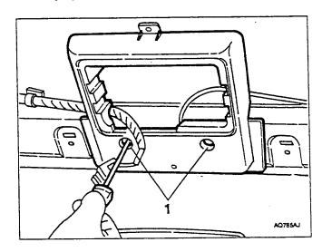
1. Release the rear courtesy light with a screwdriver, disconnect the electrical connection and remove it.
