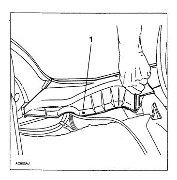
1. Using tool 1.823.014.000, prise the rear heelboard and remove it.
