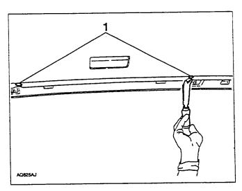
1. Lower the rear section of the roof panel trim enough to cut the glue as illustrated.
