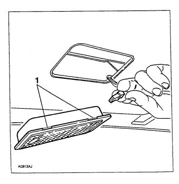
1. Slacken the two roof panel trim front fastening screws.
