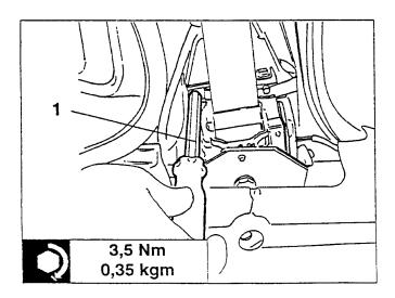
1. Separate the inner bracket from the retainer pin on the innertia reel to "disable" the pretensioner, then remove it from the pillar.
