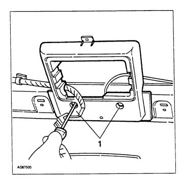
1. Release the courtesy light using a screwdriver in the two notches on the frame to free the catches, disconnect the electrical connector and remove the light.
