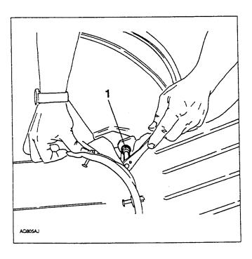
1. Remove the seat back fastening screw.
