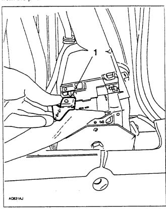
1. Through the special window make sure that the security device has been engaged checking that the spring shown by the arrow has returned to the rest position (towards the inside of the car); if not, suspend the procedure and be very careful because the device may be triggered.
