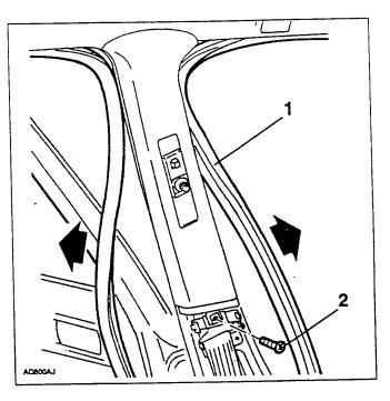
1. Using tool 1.823.014.000, prise the upper pillar cover and remove it complete with the sliding plate.
